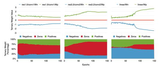
Ternary weights value (above) and distribution (below) with iterations for different layers of ResNet-20 on CIFAR-10.
