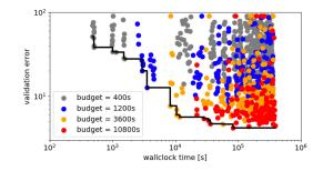
**Figure 1:** Validation error of all configurations evaluated on the different budgets during the whole optimization procedure. The best performing configuration (incumbent) as a function of time is visualized by the black line.
