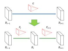
Figure 2: Network morphism linear.  $B_*$  represents blobs (hidden units), G and  $F_*$  are convolutional filters (weight matrices) for DCNNs (classic neural networks). G is morphed into  $F_l$  and  $F_{l+1}$ , satisfying Equation (6).
