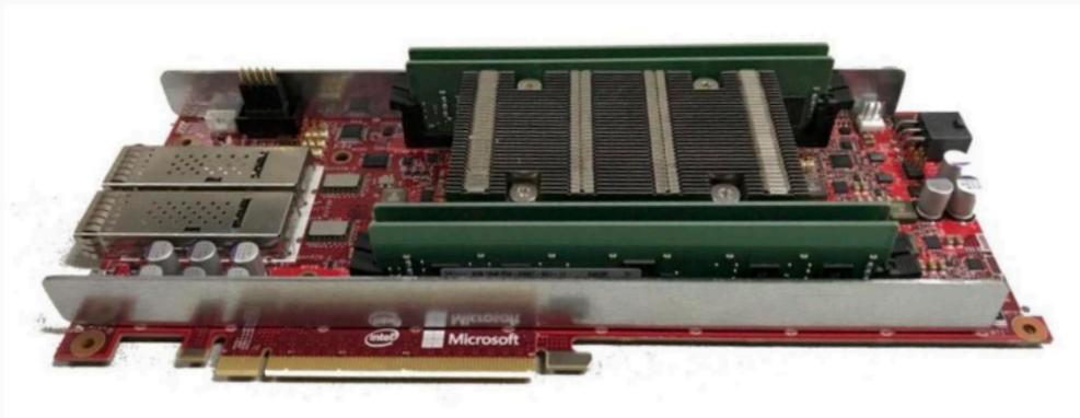
The Microsoft Brainwave mezzanine card extends each server with an Intel Altera Stratix 10 FPGA accelerator, synthesized to act as a "Soft DNN Processing Unit," or DPU, and a fabric interconnect that enables datacenter-scale persistent neural networks. MICROSOFT
