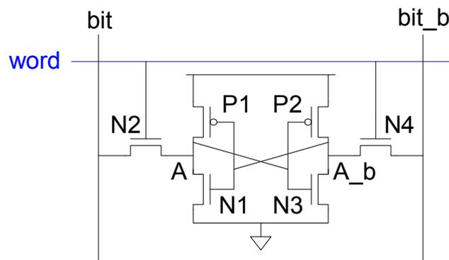
Figure 2: 6T-SRAM cell structure.
