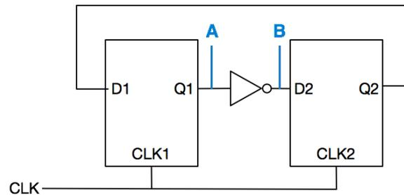
(b) In the above circuit, currently there is already one delay gate with delay  $TG$ . How many more similar delay gates can you insert between A and B without creating error?
