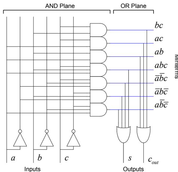
Figure 1: The Logic Circuit for Question 3
