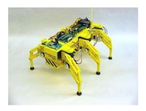
Servo motors for making robot legs http://www.lynxmotion.com/
