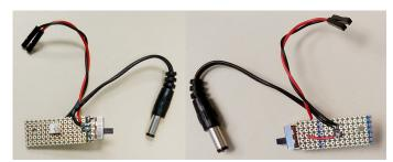
Figure 2: Power switch board.
