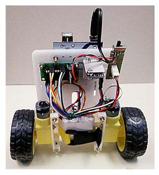
Figure 1: CENG4480 self-balancing robot.
