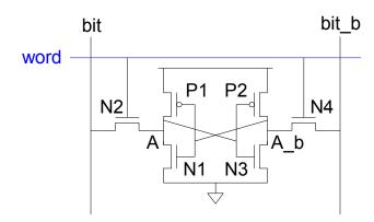
Figure 1: 6T-SRAM cell structure.
