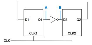
(b) In the above circuit, currently there is already one delay gate with delay TG. How many more similar delay gates can you insert between A and B without creating error?
