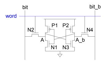
Figure 1: 6T-SRAM cell structure.
