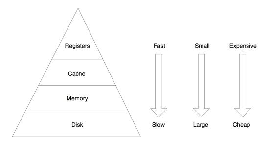
1. On-Chip Register; L1, L2 Cache; Main Memory; Secondary Storage (Disk).
