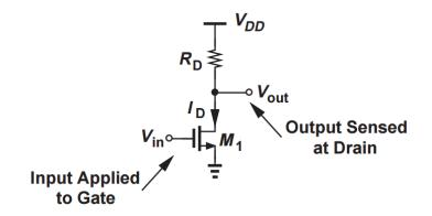
Figure 7: Common Source Amplifier
