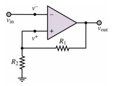
Figure 5: Schmitt Trigger
