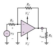
Figure 6: Inverting Amplifier
