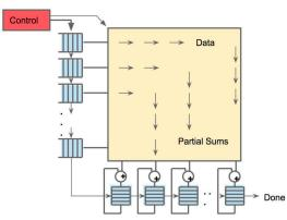
**Figure 4.** Systolic data flow of the Matrix Multiply Unit. Software has the illusion that each 256B input is read at once, and they instantly update one location of each of 256 accumulator RAMs.
