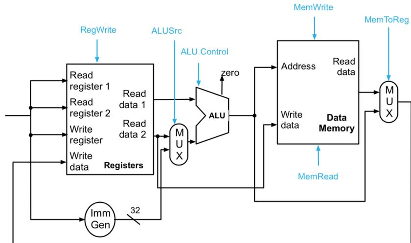
Figure 3: The datapath for the memory instructions and the R-type instructions.
