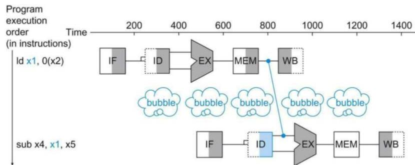
Figure 2: We need a stall even with forwarding when an R-format instruction following a load tries to use the data
