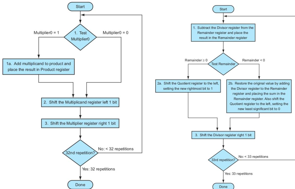
Figure 1: The left figure is the multiplication algorithm for reference. The right figure is the division algorithm.
