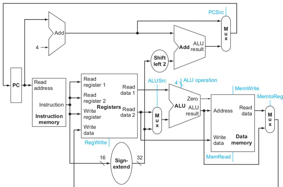
Figure 1: The datapath for the core RISC-V architecture combines the elements required by different instruction classes.
