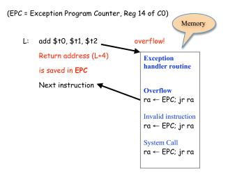
The Exception Handler determines the cause of the exception by looking at the exception code bits. Then it jumps to the appropriate exception handling routine. Finally, it returns to the main program.
