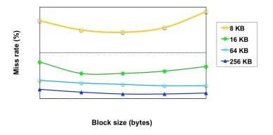
Miss rate goes up if the block size becomes a significant fraction of the cache size because the number of blocks that can be held in the same size cache is smaller (increasing capacity misses)
