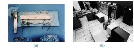
(a) 1958, by Jack Kilby@Texas Instruments, by hand. Several transistors, resistors and capacitors on a single substrate. (b) IBM System/360, 2MHz, 128KB – 256KB.
