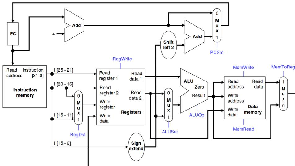
4. Based on the above datapath, finish the blanks in the following table. Here `lwd` is a new instruction. `lwd $rd, $rt($rs)` sets register `$rd` to the value at `Mem[$rs + $rt]`.
