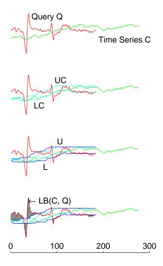
Figure 4: An illustration of the SWM envelopes. From top to bottom: A time series C and a query Q; The series C bounded from above and below respectively by UC and LC, the envelope for scaling; The series UC bounded above by U and LC bounded below by L, forming the overall envelope for scaling and time warping; and the lower bounding distance LB derived from the overall envelope.
