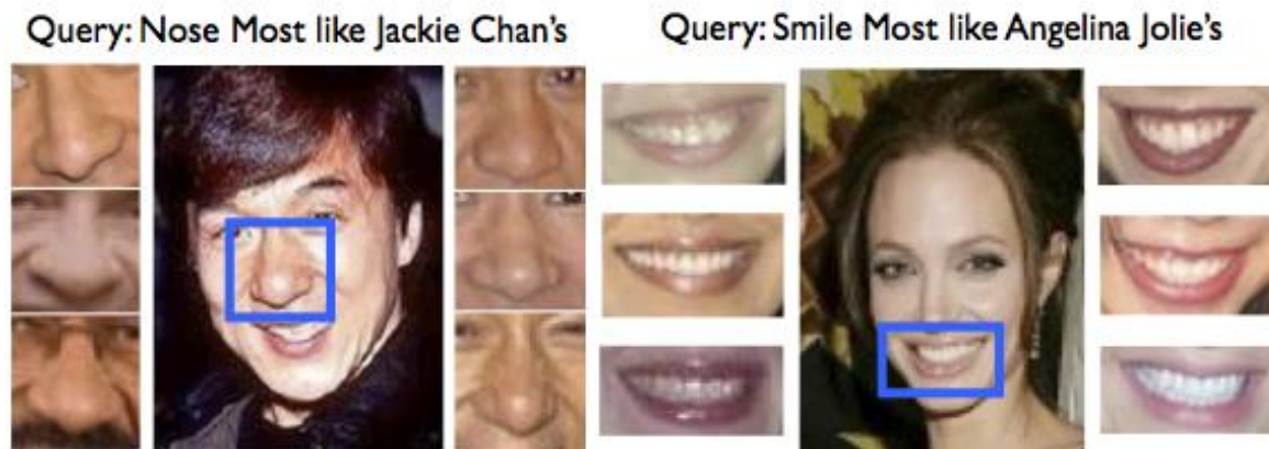
Figure 3 [16]: Searching for local feature (nose and smile) matches of images. Same technique can be applied to search for matches of the entire image as a whole by including multiple local features.
