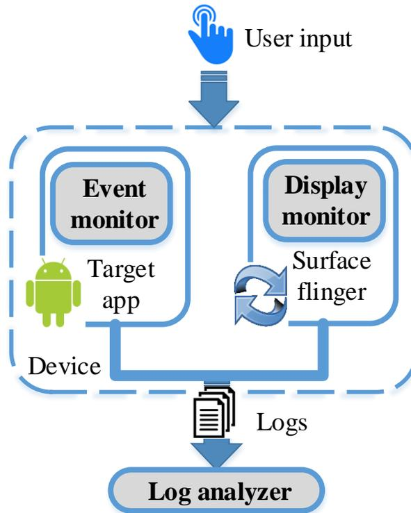
Figure 4.5: Detecting poor-responsive operations
