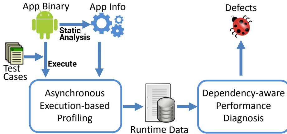
Figure 3.5: Overview of DiagDroid Framework
