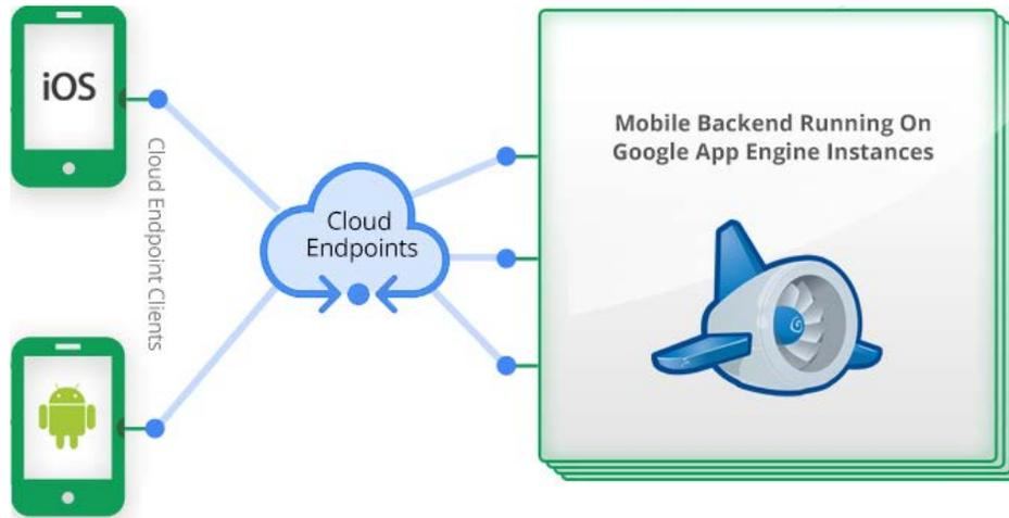
Figure 1.2: Google cloud endpoints & app engine architecture
