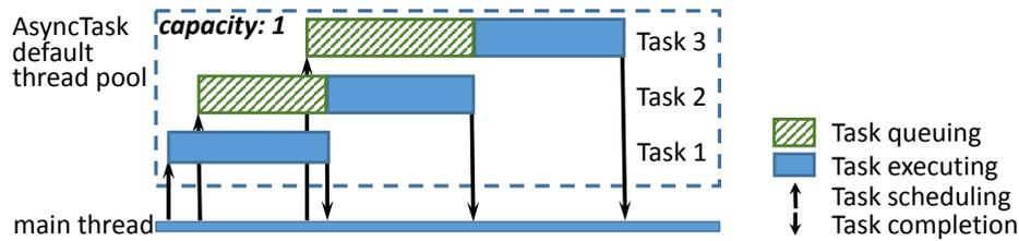
Figure 3.6: Asynchronous tasks runtime
