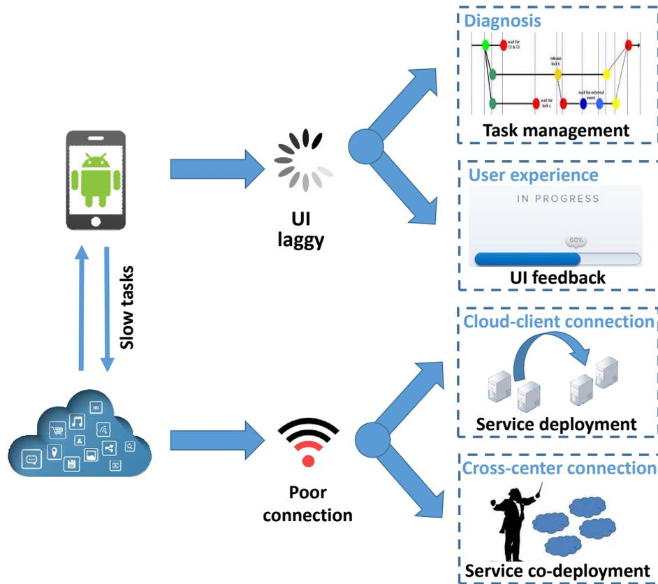
Figure 1.3: An overview of cloud-based mobile app performance tuning
