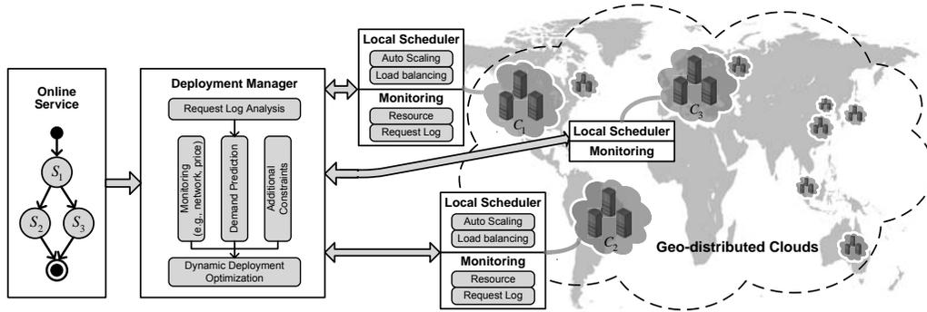
Figure 3.6: The Framework of Service Deployment in Geo-distributed Clouds
