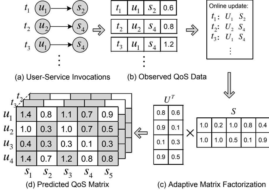
Figure 4.3: An Example of QoS Prediction by Adaptive Matrix Factorization
