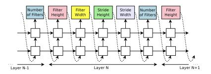
Figure 2.10: Recurrent neural network for the RL controller to search convolutional neural networks [3].
