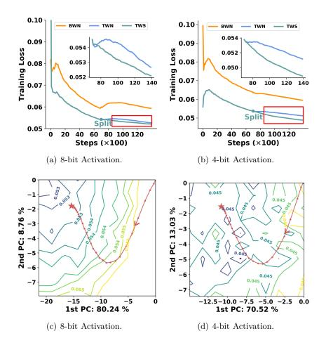
Figure 5.8: (a) and (b) show the training curves on MRPC under different activation bits. The red box is enlarged in the sub-figure. (c) and (d) visualize the fine-tuning trajectories after splitting, on the 2-D loss contour of BinaryBERT.
