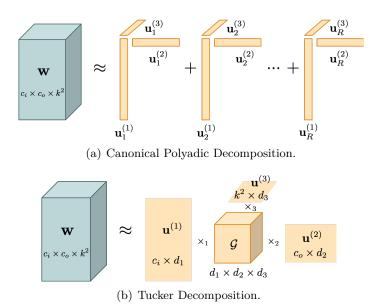
Figure 2.6: Two common tensor factorization approaches: (a) Canonical Polyadic (CP) decomposition, and (b) Tucker decomposition for tensor parameters.
