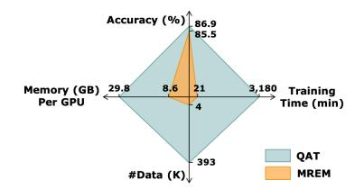
Figure 4.1: An illustrative comparison between our parallel post-training quantization method (MREM) and QAT on four dimensions. The results are based on a quantized BERT-large model with 4-bit weights and 8-bit activations over the MNLI dataset. Best viewed in color.
