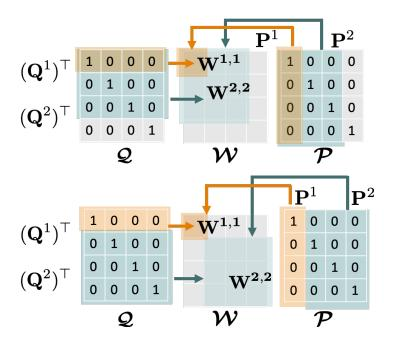
Figure 6.3: A 2-dimensional illustration of affine parameter sharing with ordinal selection (up) and independent selection (down). The candidate kernel is constructed by transforming the meta-weights into proper shapes with two transformation matrices.
