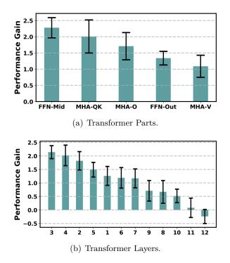
Figure 5.5: The performance gain of different Transformer parts and layers in descending order. All numbers are averaged by 10 random runs with standard deviations reported.
