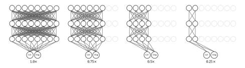
Figure 2.12: An illustration of parameter sharing from [5]. The four choices of widths are ordinally overlapped along channel indices.
