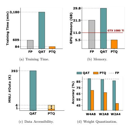
Figure 4.2: Comparison between QAT and PTQ over four dimensions. We use a BERT-large model over MNLI dataset for illustration. The full-precision (FP) fine-tuning is also included as a baseline. We follow the procedure in [6] for QAT, and REM in Equation (2.11) for PTQ. The training time and memory in (a) and (b) are measured by 4-bit weights and 8-bit activations (i.e., W4A8) on an NVIDIA V100.
