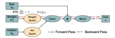
Figure 2.3: The computational graph of a quantized convolutional neural network. The rectangles and circles denote the intermediate tensors and operations respectively. The forward pass first quantizes tensors into the convolutional operation. In the backward pass, the STE operator copies the gradient  $\nabla \ell(\hat{\mathbf{w}})$  of quantized  $\hat{\mathbf{w}}$  directly to  $\mathbf{w}$ .
