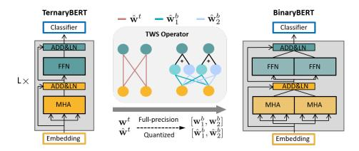
Figure 5.4: The overall workflow of training BinaryBERT. We first train a half-sized ternary BERT model, and then apply ternary weight splitting operator (Equations (5.6) and (5.7)) to obtain the latent full-precision and quantized weights as the initialization of the full-sized BinaryBERT. We then fine-tune BinaryBERT for further refinement.
