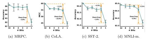
Figure 5.1: Performance of quantized BERT with varying weight bit-widths and 8-bit activation. We report the mean results with standard deviations from 10 seeds on MRPC, CoLA, SST-2, and 3 seeds on MNLI-m, respectively.
