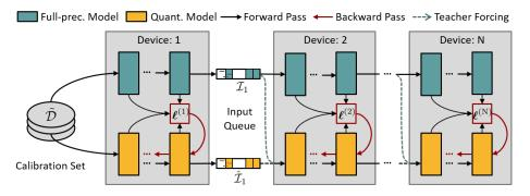
Figure 4.3: The overview of the proposed module-wise reconstruction error minimization (MREM). We partition both the full precision model and quantized model into multiple modules on different computing devices. By collecting tensors from the input queue, MREM can be conducted locally without waiting for the predecessor. Teacher forcing can be applied to mitigate the issue of reconstruction error propagation.
