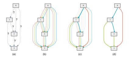
Figure 2.9: The overview of differentiable neural architecture search (DARTS) from [2]. (a) shows the initialized network with unknown operations; (b) shows the continuously relaxed architecture parameters for different connections among cell nodes; (c) illustrates the searching process with preferred operations being thicker; In (d) the operations with the highest probability for each connection are picked to finalize the architecture.
