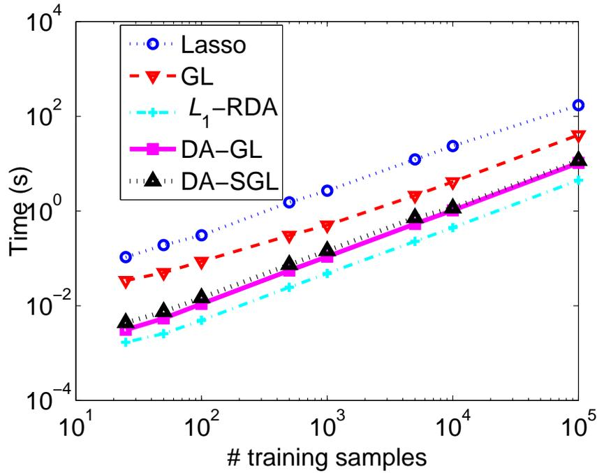
Figure 3.1: Log-log plot of computation time on training the synthetic dataset. The batch-model algorithms suffer from much time cost in loading large-scale datasets.
