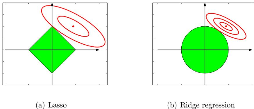
Figure 2.3: Illustration of solutions on the lasso and ridge regression.
