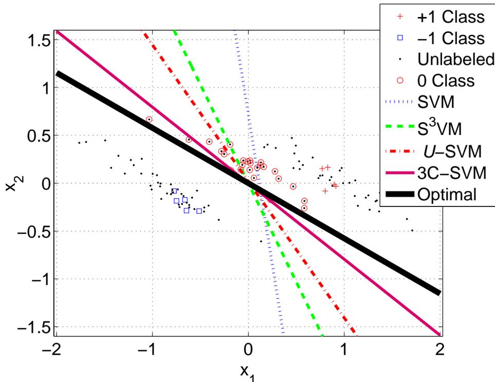
Figure 5.2: Illustration of different classifiers in  $\mathbb{R}^2$  space. The 3C-SVM (the thin solid line) achieves the best result, which is closest to the Bayesian optimal classifier (the thick solid line), among all other maximum margin classifiers and automatically distinguishes the irrelevant unlabeled data (black dots with red circles) correctly.
