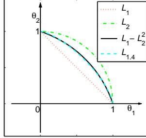
Figure 6.1: Demonstration of a linear combination ( $v = 0.5$ ) of the  $L_1$ -norm and the squared  $L_2$ -norm on  $\boldsymbol{\theta}$  in  $R^2$  space. Although,  $L_p$ -norm ( $p = 1.4$ ) can obtain a similar curve to that of the linear combination of the  $L_1$ -norm and the squared  $L_2$ -norm, it produces non-sparse solutions.
