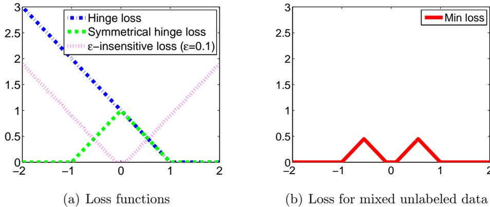
Figure 5.3: Illustration of loss functions. The min loss is the minimum between the symmetrical hinge loss and the  $\varepsilon$ -insensitive loss.
