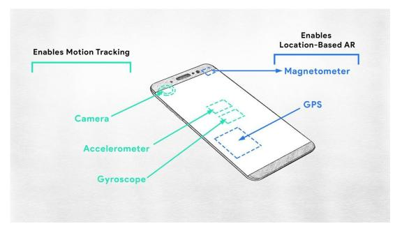
Figure 5-3 Hardware of mobile phone enhancing the motion tracking
