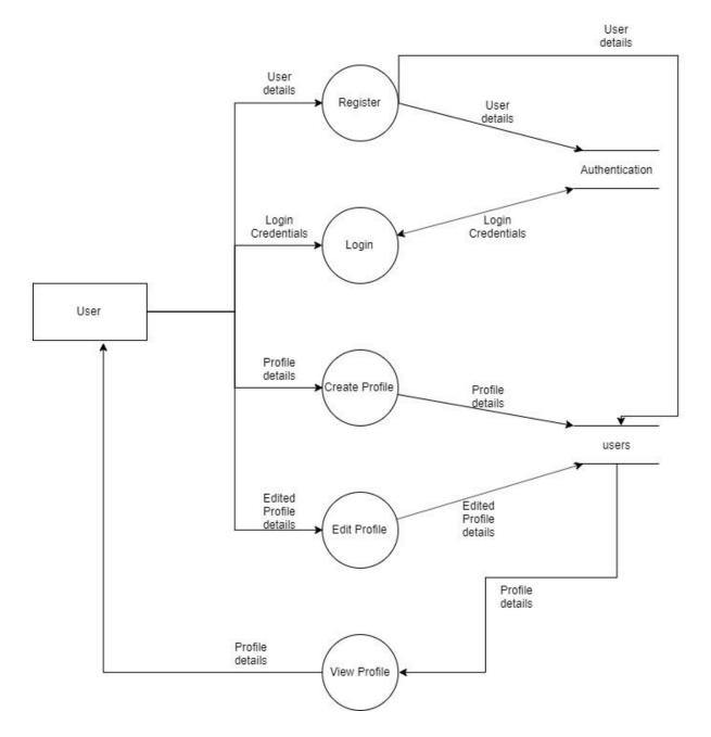
Fig. 3.5.1.1 Authentication and profile system data flow diagram
