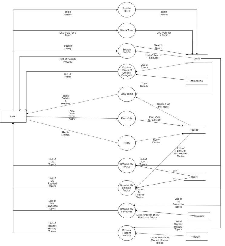
Fig 3.5.2.1 Main system data flow diagram
