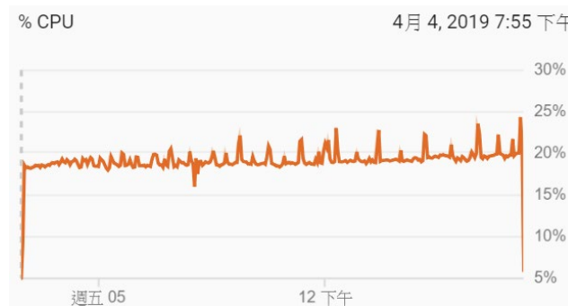
Figure 5-19: CPU usage graph of 1000000 ballots test
