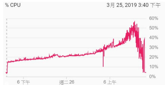
Figure 5-7: CPU usage graph of 1000000 ballots test on Google VM
