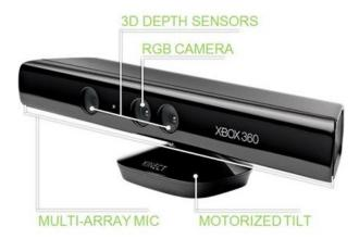
Figure 2.3 Kinect structure
