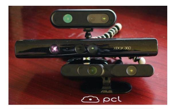
Figure 3.7 Kinect device
