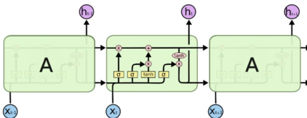
Figure 10: LSTM layer structure
