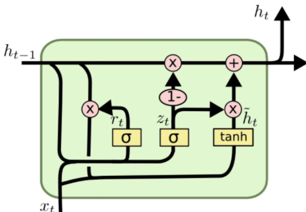
Figure 11: Structure of a GRU unit
