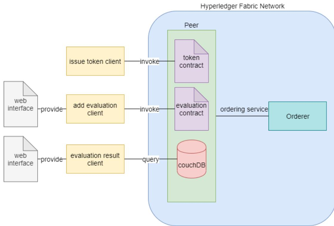
Figure 14: System architecture diagram of blockchain network [18]
