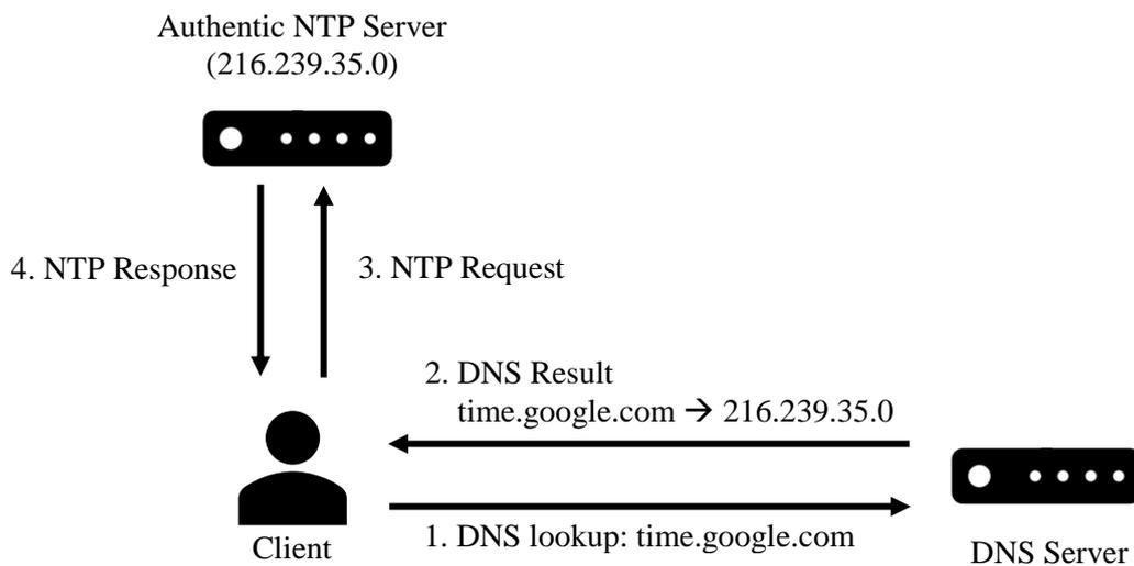
*Figure 2.4 NTP Time synchronization in an expected environment. Client has NTP server configured to time.google.com is resolved correctly to the authentic NTP server.*
