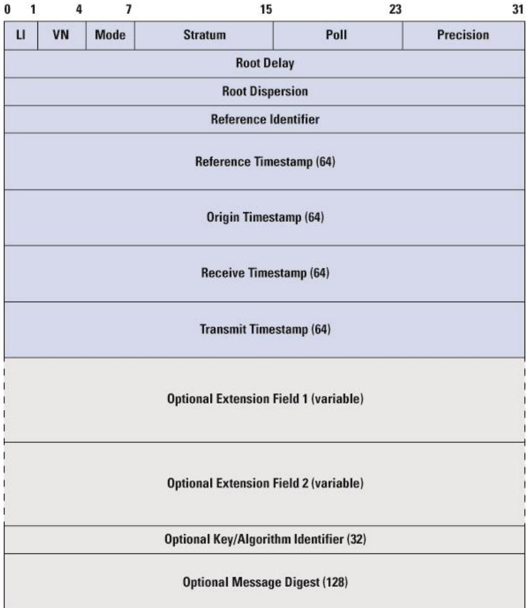
*Figure 2.2 NTP Packet Format*
