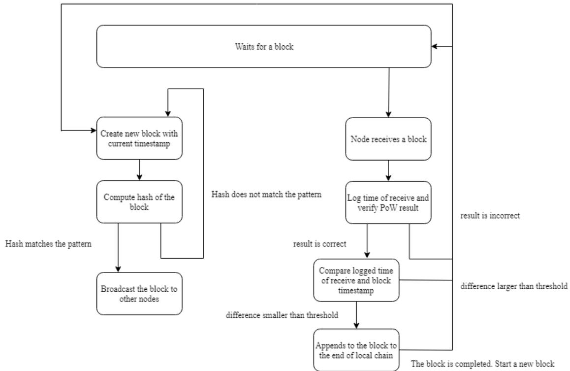
Figure 3.4 Flow of Timechain
