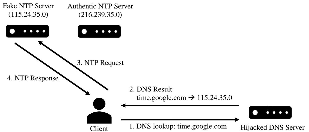
Figure 2.5 The DNS server is hijacked and time.google.com is resolved to another address. The client hence requests the NTP time from the fake server without authenticating and update its own time accordingly.
