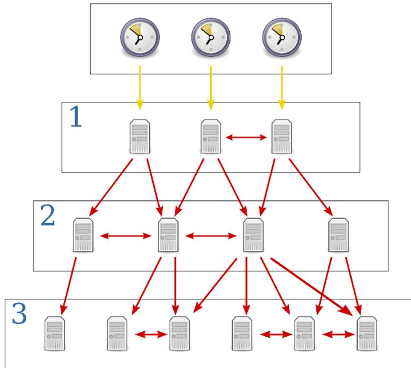
*Figure 2.1 Illustration of NTP Connections*
