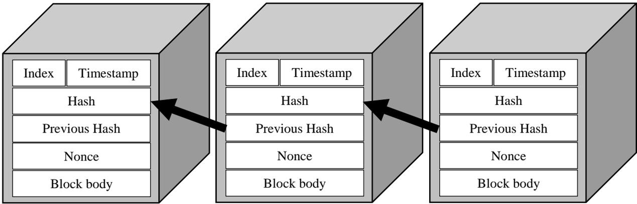
*Figure 3.1 Illustration of relationship between blocks*
