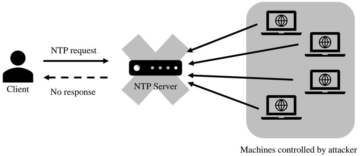
*Figure 2.6 Illustration of attacker disabling NTP server with big volume of requests.*
