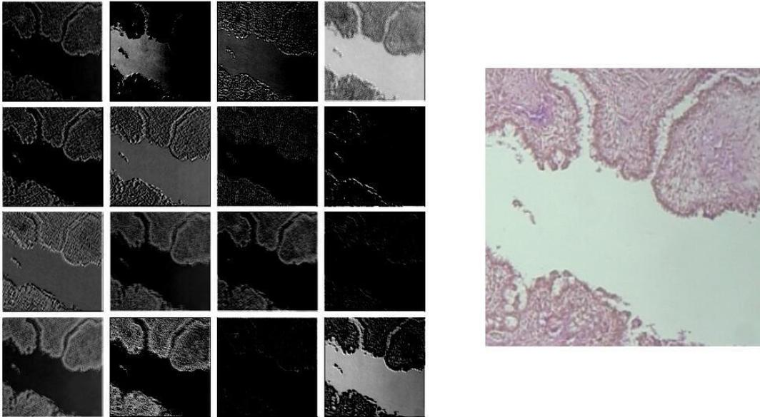
Figure 7.6 feature maps learned by first convolution layer, right side is the raw data and left side is 16 feature maps the model learned
