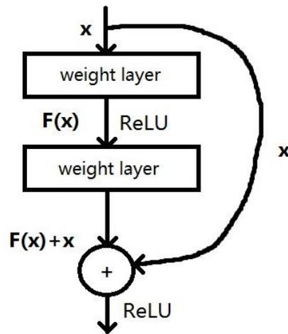
Figure 5.8 A Simplified Residual Block
