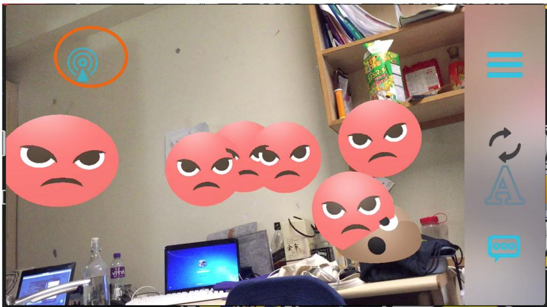
The above view is showing that beacon is adopted, when there is registered beacon nearby, instead of using GPS, beacon will be immediately choosing as the position system. The transparency of icon is indication the signal strength of beacon. There is 3 level, far,
