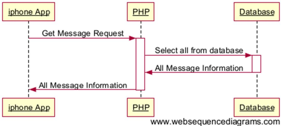
The above sequence diagram is showing how the message is get from the database. The app first sends a http request to server, via the PHP send a SQL command to database to retrieve all the message information. The messages will send back to app via the PHP by an http response. The above get message procedure will be invoked when map view is pull to the foreground.
