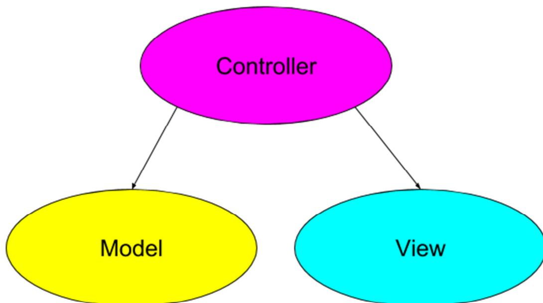
MVC is an object-oriented design pattern. Model object is defining the data and logic that manipulates that data. View object is presenting information and getting user input. Controller is performing set-up and coordinating tasks among model object and view object.
