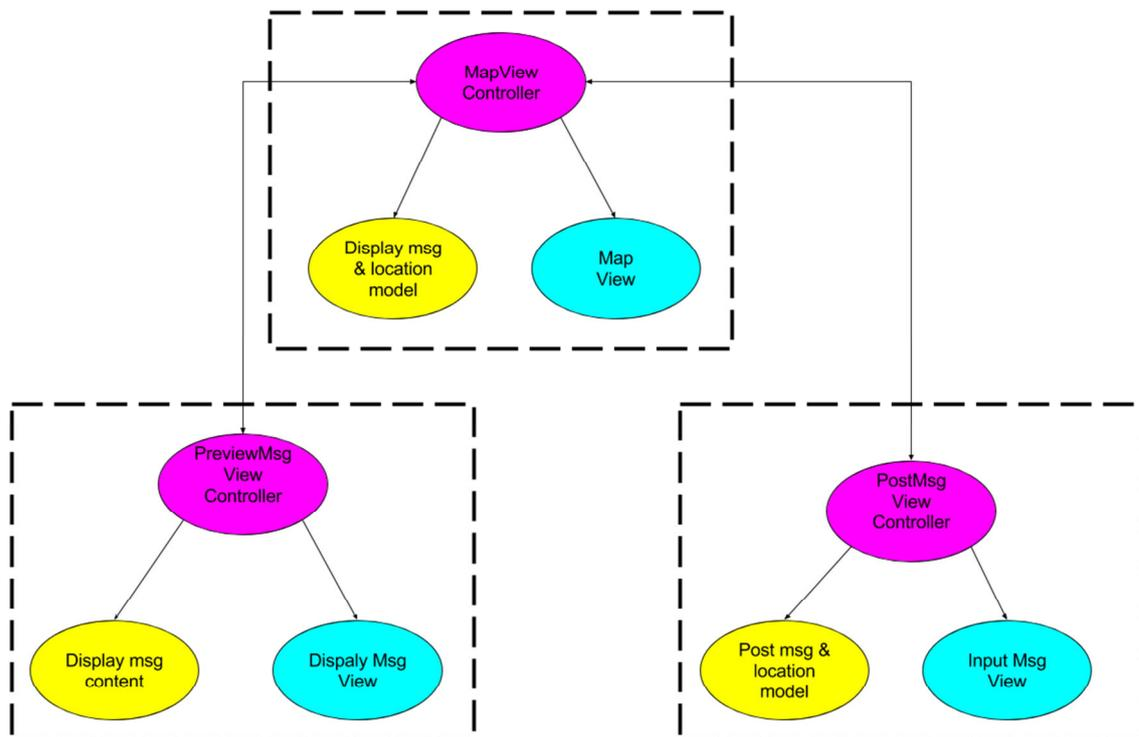
The above diagram is showing the MVC model of our app. They are divided into three modules, Map View, Preview Message View and Post Message View. Each controller is having different or same model object to serve for the purpose of that view.
