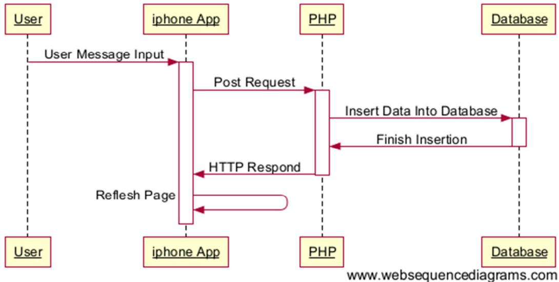
The above sequence diagram is show how the message being post to database. User input message and choose tag, after pressing the submit button, the app send a http post request with message information to the server, via the PHP a SQL insert command is send to database. Then the server will send back http respond to indicate the message is successfully upload. The app then refreshes the page to map view, the get message procedure will immediately invoked to update message information.
