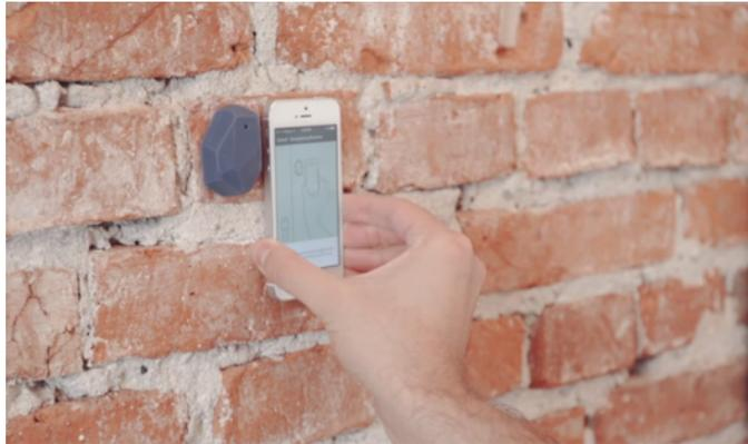
**Figure 7:** The developer is mapping his room to Estimote Cloud using the Estimote Indoor Location app. [7]
