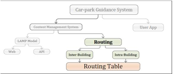
Figure 5.3.1 – Routing of Car-park Guidance System
