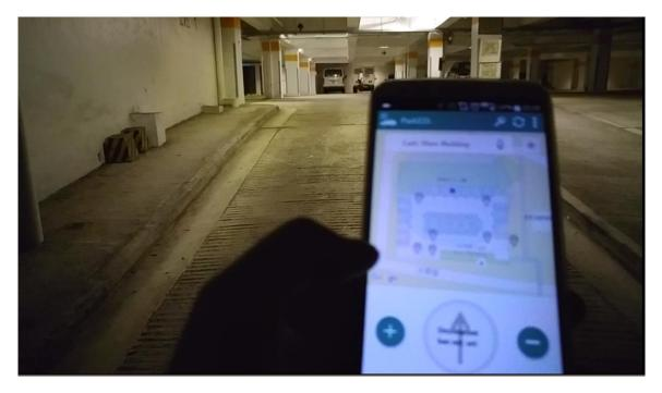
2. User App detects the Beacon signal which installed near to the entrance of LSB car park. And show "car icon" on the map to indicate my physical location on floor plan.
