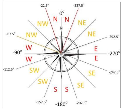
Figure 5.5.13 – Degree (Sensor Reading) to Absolution Direction conversion
