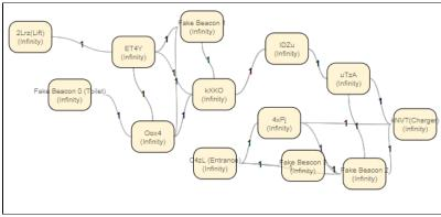
Figure 5.1.14 – Example of Topology of Beacon Network
