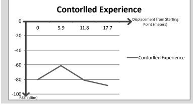
Figure 4.1.7 – RSSI against Displacement graph (Controlled Experience Result)
