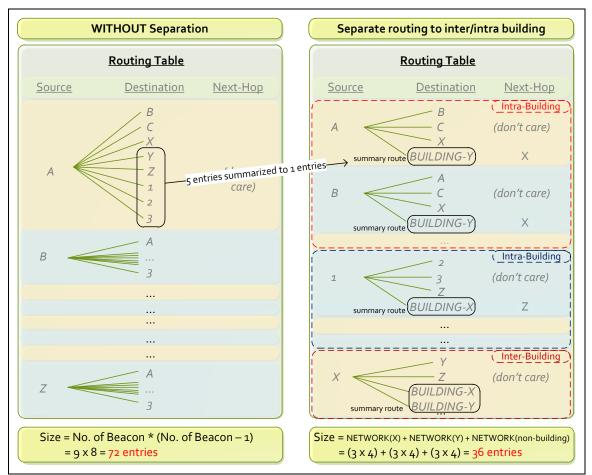
Figure 5.3.6 – Routing Tables Comparison (Separate vs. Without Separate)
