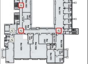
Figure 7.1.3 – Beacon Deployment on 10/F
