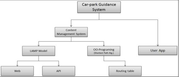
Figure 5.1.2 – Architecture of Content Management System
