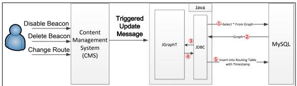
Figure 5.4.11 – Triggered Updated Approach to build routing table
