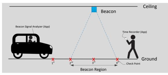
Figure 4.1.1 – The Setup of Time Delay Error Experience
