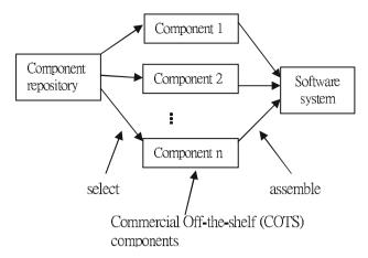
Fig. 1. Component-based software development.
