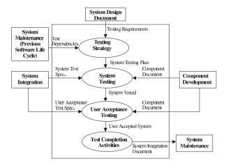
Fig. 10. System testing process overview.
