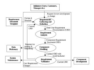
Fig. 4. Component requirement analysis process overview.
