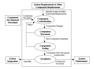
Fig. 7. Component customization process overview.
