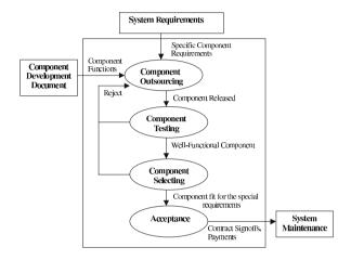
Fig. 6. Component certification process overview.
