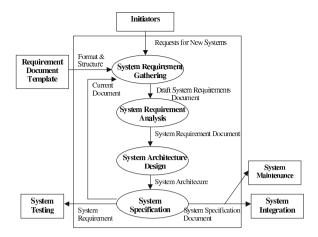
Fig. 8. System architecture design process overview.
