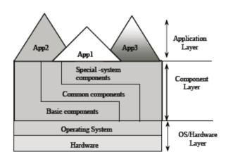
Fig. 2. System architecture of component-based software systems.
