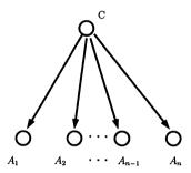
Fig. 1. A Naive Bayesian Classifier.  $A_i, 1 \le i \le n$ , is the attribute. In this figure, the attribute is independent of each other, given the class label C.
