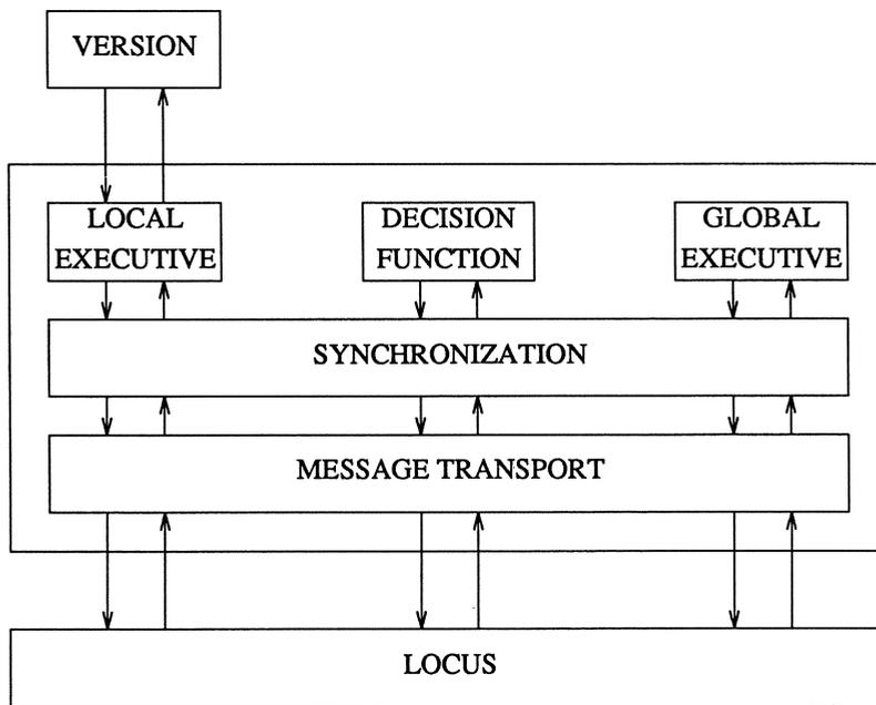
Fig. 3. The Standard DEDIX Configuration on One Site
