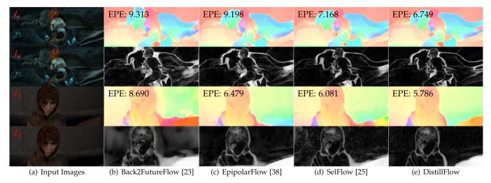
Fig. 6. Qualitative comparison with state-of-the-art unsupervised learning methods on Sintel Final benchmark. For each case, the top row is optical flow and the bottom row is error map. The whiter the color in the error map, the greater the error. More examples are available on the Sintel benchmark.
