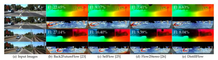
Fig. 5. Qualitative comparison with state-of-the-art unsupervised learning methods on the KITTI 2015 benchmark. For each case, the top row is optical flow and the bottom row is error map. The redder the color in the error map, the greater the error. More examples are available on KITTI 2015 benchmark.
