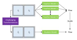
Fig. 1. Framework illustration. We distill confident optical flow estimations from teacher models (stage 1) to guide the flow learning of the student model (stage 2) under different challenging transformations.
