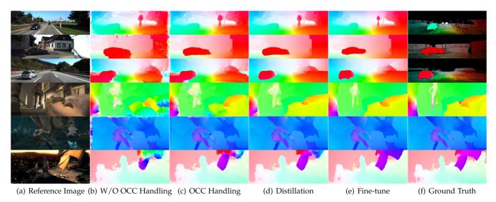
Fig. 7. Ablation study on KITTI 2015 (top 3) and Sintel Final training datasets (bottom 3). (b) and (c) are the results of without and with occlusion handling. (d) shows that results with knowledge distillation and (f) is the supervised fine-tuned results. With knowledge distillation, the flow looks more smooth. After fine-tuning, more details are preserved. Zoom in for details.
