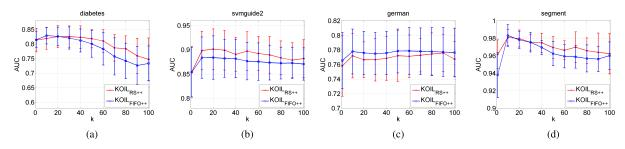
Fig. 4. Average AUC of the KOIL algorithm with different k values. Here, k = [1, 10:10:100] and the budget is 100 for each buffer.
