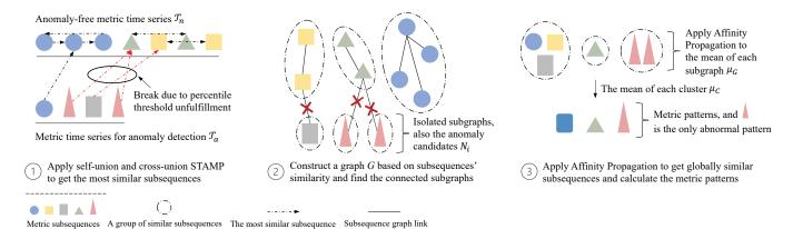
Figure 3: The Algorithm of Performance Anomaly Pattern Discovery
