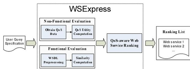
**Figure 2. System Architecture**
