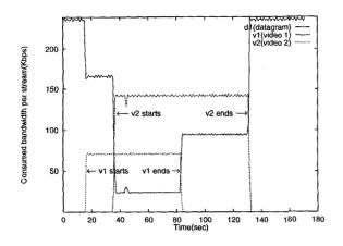
Fig. 2. Channel bandwidth usage, with QoS support
