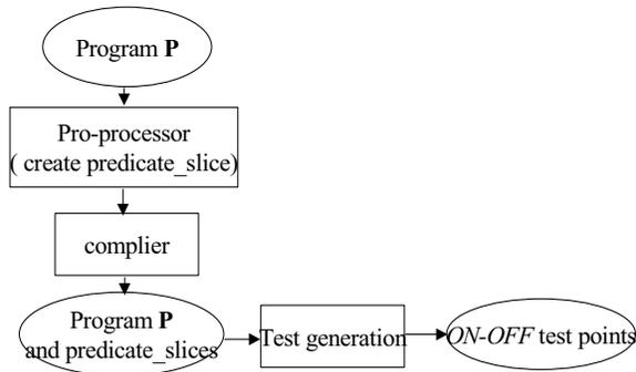
Fig.3 The architecture of automatic test generator
