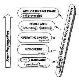
Figure 1. Layered software architecture model.
