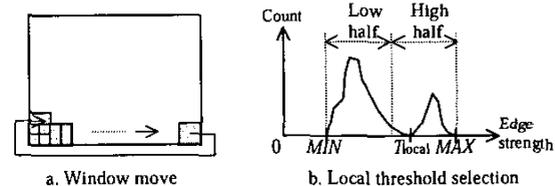
Figure 4. Local thresholding
