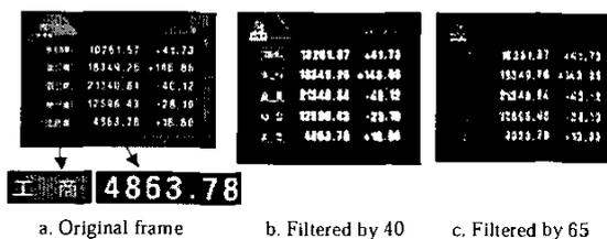
Figure 1. Different contrast of texts in one frame
