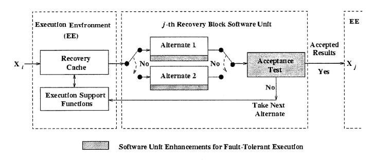
Figure 6 The Recovery Block (RB) Model
