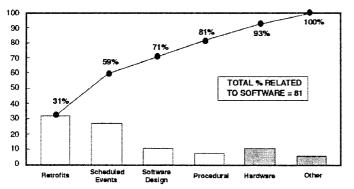
Figure 1 Switching System Outage Causal Classification
