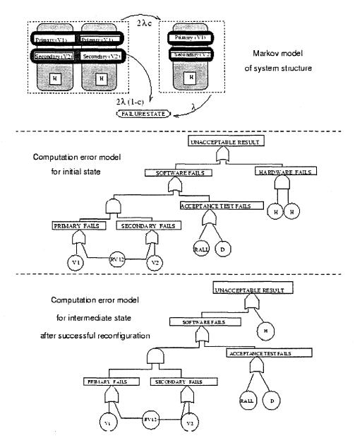
Figure 3 Fault Tree Analysis for Fault Tolerant Software
