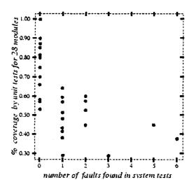
Figure 9 Relationship of Unit Coverage Testing to System Test Faults for One System
