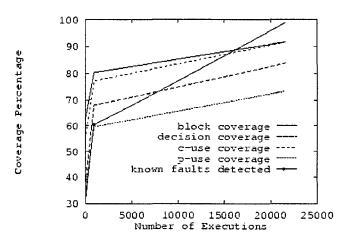
Figure 8 Relationship between Coverage Improvement and Fault Detection during Testing Phases
