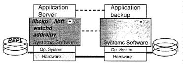
Figure 4 Software Fault Tolerance: Platform and Components
