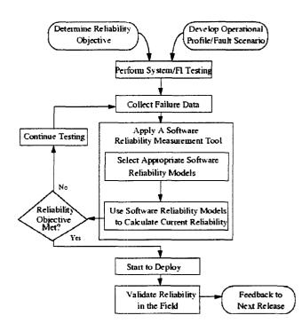
Figure 10 Software Reliability Measurement Procedure
