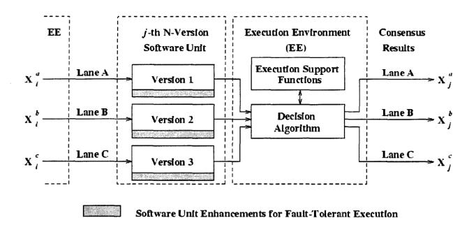
Figure 5 The N-Version Software (NVS) Model with N = 3
