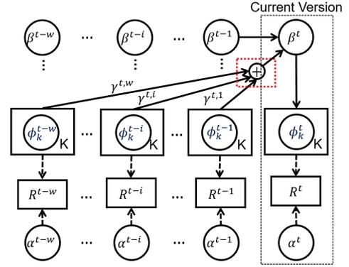
**Figure 5: Overview of AOLDA.** The red rectangle with dashed dots highlights the adaptive integration of the topics of the  $w$  previous versions for generating the prior  $\beta$  in the  $t$ -th version.  $R^t$  is the review corpus in the  $t$ -th version. The dotted lines indicate that we simplify the original LDA [4] steps for clearness.
