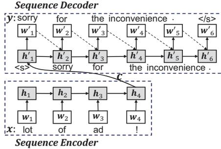
Fig. 2: An overall architecture of RNN encoder-decoder model.
