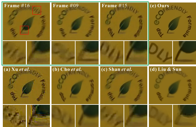
Figure 1. Multi-frame super-resolution (SR) results on a real video sequence. Green box: Input frames ( 150 \times 120 ) directly cropped from a video captured by an iPhone. Three clearest frames are shown. Motion blur and compression artifacts are present. (a) Result of single image deblurring [30]. (b) Result of video deblurring [7]. (c) Result of video upsampling [19]. (d) MFSR result [16]. (e) Our result ( \times 3 ).
