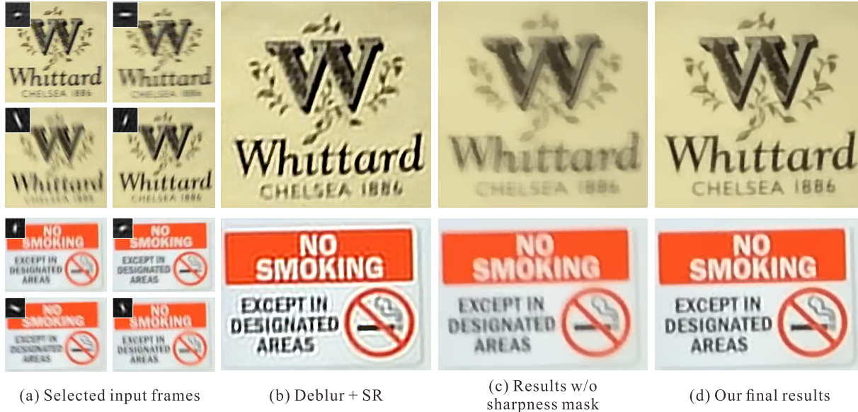
Figure 7. More results and comparison ( \times 3 ). (a) Four input frames from each sequence. (b) Results of multi-image deblurring [32] followed by super-resolution [16]. (c) Results without sharpness mask ( \beta = \infty ). (d) Our results with the sharpness masks ( \beta = 1.4 ).
