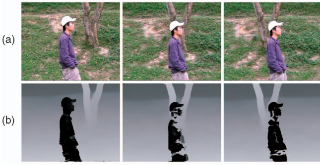
Fig. 2. Depth recovery with dynamic objects. (a) Selected frames from an input video. (b) Recovered depth maps. Although the depth estimates for the dynamic foreground are problematic, they do not much affect the background depth estimation.
