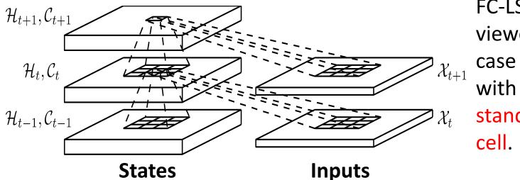
FC-LSTM can be viewed as a special case of ConvLSTM with all features standing on a single cell.
