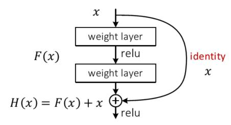
H(x) is any desired mapping, hope the 2 weight layers fit H(x)hope the 2 weight layers fit F(x)let H(x) = F(x) + x
